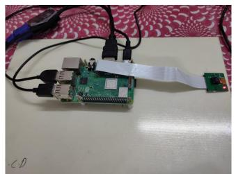
Fig 5 Kit and Pi camera connection
