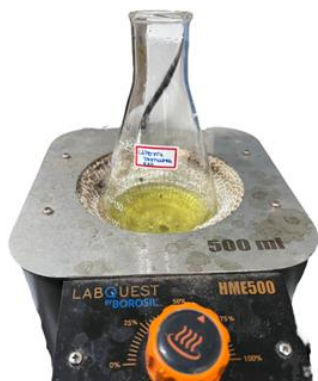
Figure 1 illustrates Boiling of extract for 10-15mins at 40 degrees Celsius.
